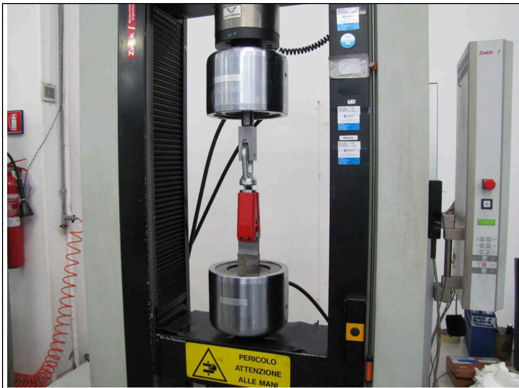
photo 2: sample "134 autoblock" – test layout
