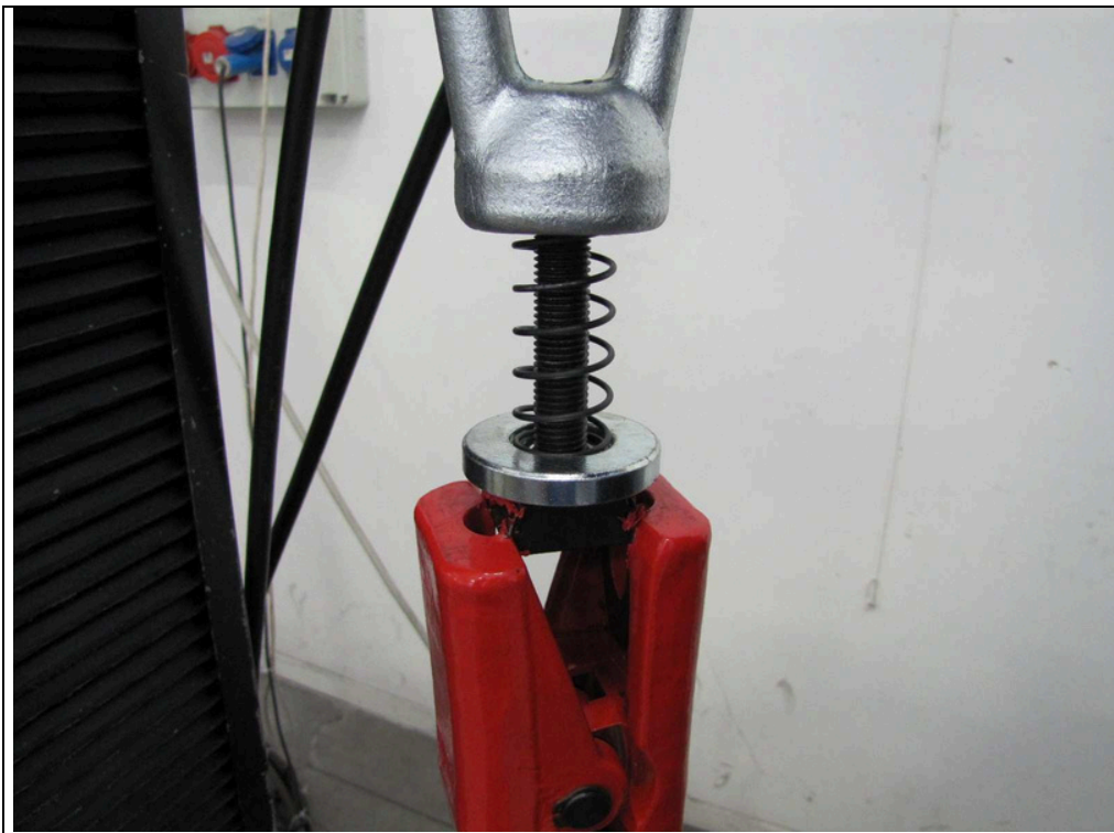
photo 3: sample "134 autoblock" – state of the device at the end of test
